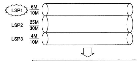
TOTAL AVAILABLE BANDWIDTH - AVAILABLE BANDWIDTH OF LSP1 = 15M - 4M = 11M, WHICH IS GREATER THAN EFFECTIVE LOAD (6M) ON LSP1. TRAFFIC CAN BE REDISTRIBUTED WITHOUT LOSS.
